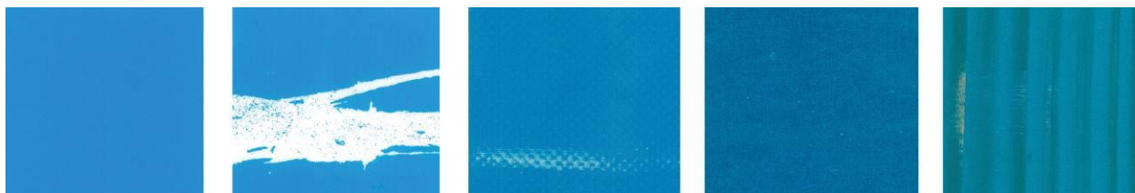
Figure 2. Visual representation of printed ink on different substrates after resistance to friction test (Paper – Plastic – Canvas – Metal – Wood)
