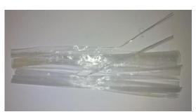
Figure 1. PP-foil type-450-tex-2223 made from pure FY-6 granulate using extrusion
