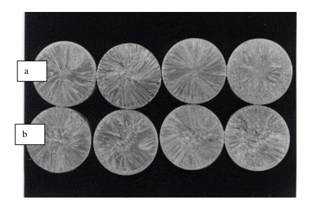
Figure 1. Macrostructure of samples 99.5% Al with different cooling rates, the top surface: a) air-cooled, b) water cooled
